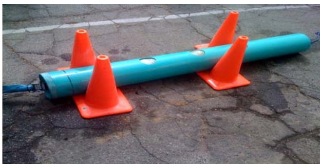
Completed cured in-place pipe liner.
