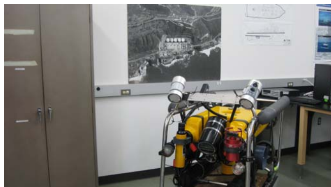
Remote diving vehicle used for video inspection of the ocean outfall.
