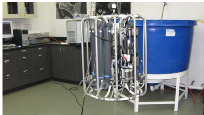
Remote sampling device used to take water samples at various depths along the ocean outfall.
